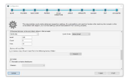
BarcodeOCR has to stipulate the threshold between white and black values in the document in order to separate the light areas in the barcode from the dark ones. There are two options for this.
